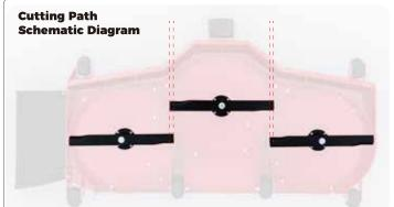
We adhere to a high-efficiency design philosophy, incorporating overlapping cutting zones between our mower blades. The overlap ratio may vary depending on the specific mower model and blade dimensions, ensuring optimal cutting performance across different operational requirements.
